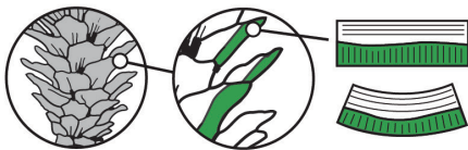
Varying response of layered materials controls shape
