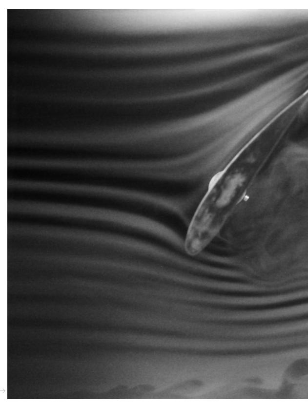
Fog (water particle) wind tunnel visualization of a NACA 4412 airfoil at a low speed flow (Re=20.000) | Photo: Georgepehli, 2010
