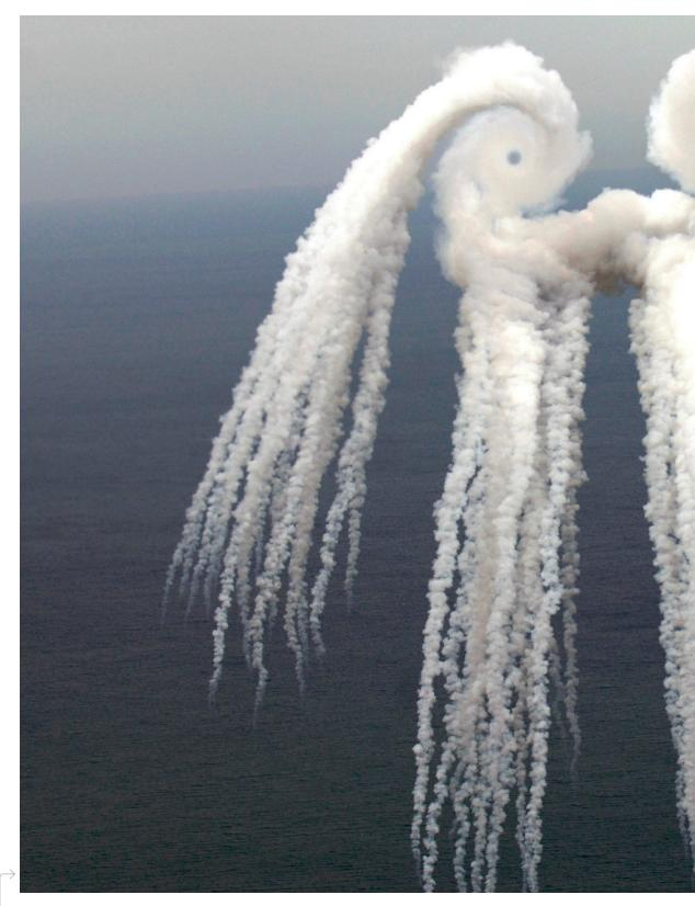
C-17 vortex: The "smoke angel" is caused by wing vortices at the plane's wingtips
