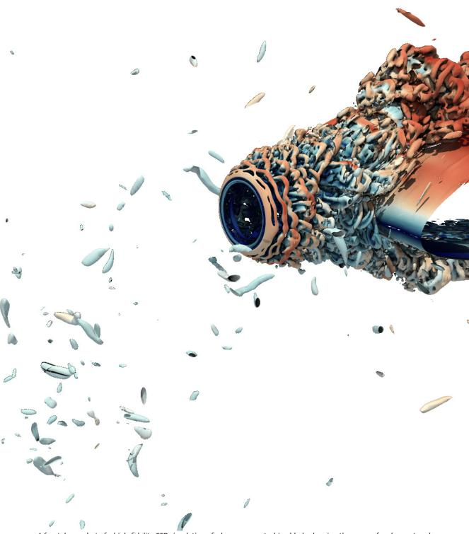
A frontal snapshot of a high-fidelity CFD simulation of a low pressure turbine blade showing the range of scales captured. Photo: Engineering at Cambridge, 2017 | Flickr cc
