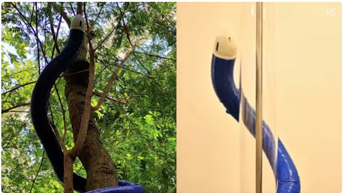
Meet FiloBot: the self-building, vine-like climbing robot Video: The New Scientist, 2024 | https://www.youtube.com/watch?v=t3aerY5gcSk
